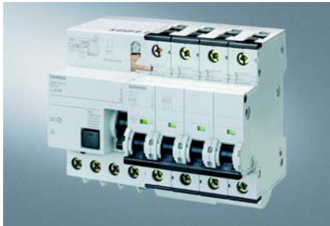
The two components are simply plugged together without the need for any tools. After the connecting screws of the conductor connection between the RC unit and the MCB have been tightened, the two devices form an RCBO.
