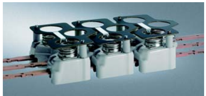
DIAZED bus-mounting base DII 3-phase for 3 x 25 A, 5SF2 07 with terminal version "B" mounted onto 3 EZR 5SH3 54 busbars. The busbars have a load capacity of 150 A each respectively.
