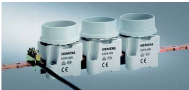
DIAZED bus-mounting base DII for 25 A, 5SF6 005 with terminal version "B" mounted onto an EZR 5SH3 54 busbar. The feeding conductors are clamped to the 8JH4 122 bus-mounting terminal. The busbar has a load capacity of up to 150 A.
